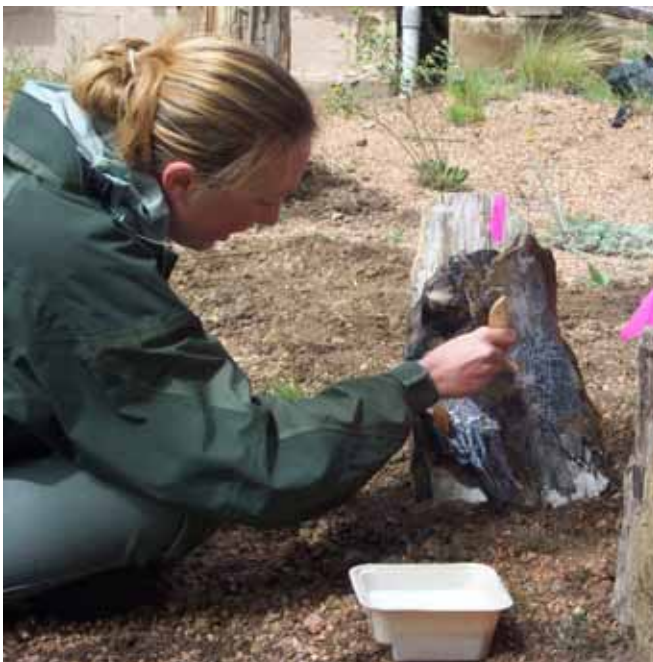
Jennifer Young, a GIP at Florissant Fossil Beds, leads an experiment to test protective coatings to minimize weathering of the petrified giant redwood stumps.
