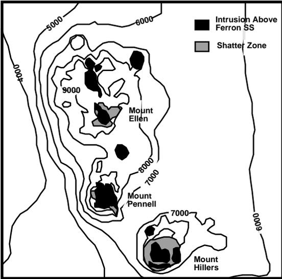
**Figure 4.** Structure contour map of the Henry Mountains. Contours drawn at the base of the Ferron Sandstone Member of the Mancos Shale. (After Hunt, Averitt and Miller, 1953)
