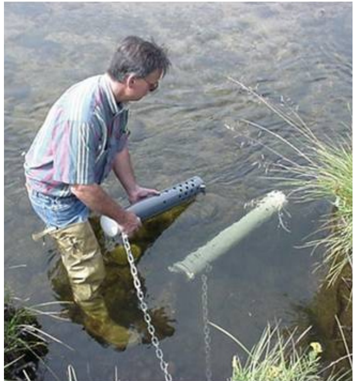
Deployment and testing of water quality data sondes at Rocky Mountain National Park.
